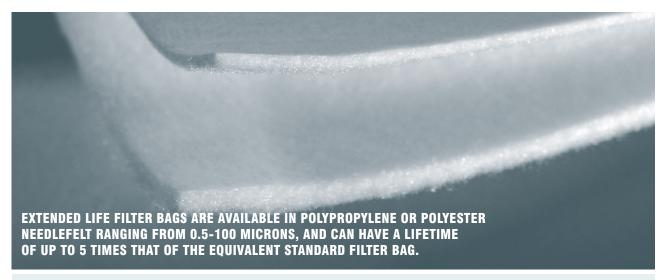
Increased thickness of the filter media compared to that of the equivalent standard felt filter bag enables an increased retention of particles. In addition, the extended life filter media has a graded density structure i.e. progressively smaller particles are captured as the fluid follows a tortuous path through the media, stopping the filter bag from blinding prematurely. The result is a filter media with a higher dirt holding capacity, leading to increased filter bag lifetime.
